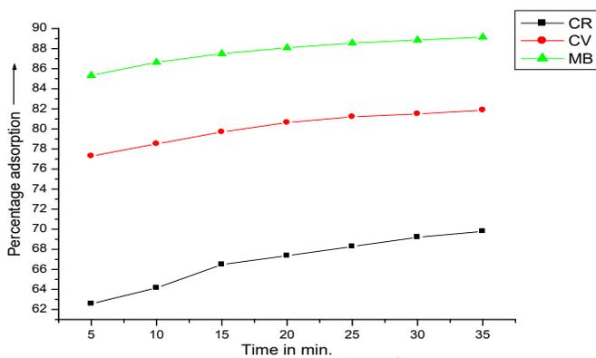
Fig.2: Comparative graph showing effect of contact time on percentage adsorption of CR, CV and MB on MSH.
