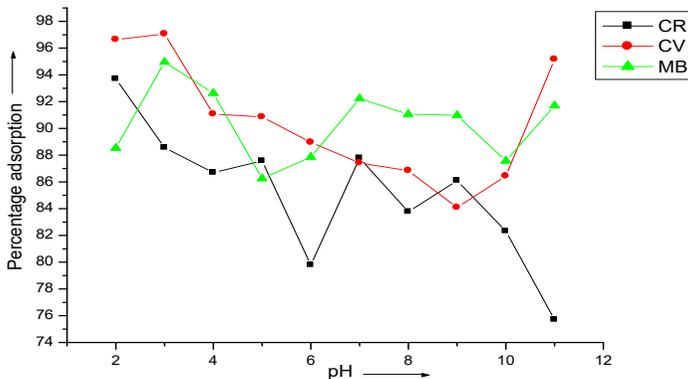
Fig.4:Comparative graph showing effect of pH on percentage adsorption of CR,CV and MB on MSH.
