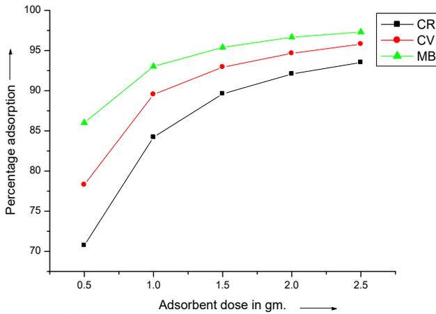
Fig.3:Comparative graph showing effect of adsorbent dose on percentage adsorption of CR,CV and MB on MSH.
