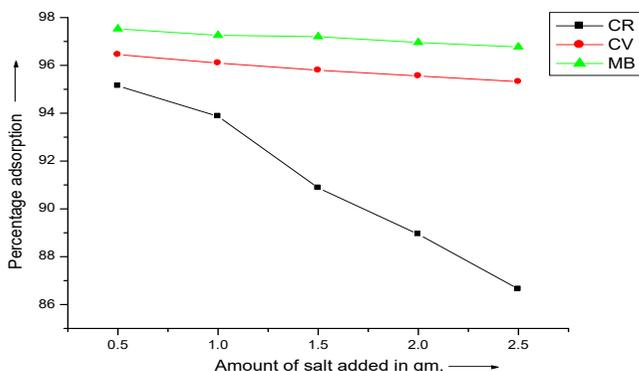
Fig.5: Comparative graph showing effect of salt added on percentage adsorption of CR,Cv and MB on MSH.
