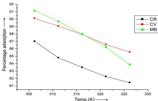
Fig.6: Comparative graph showing effect of temperature on percentage adsorption of CR,CV and MB on MSH.
